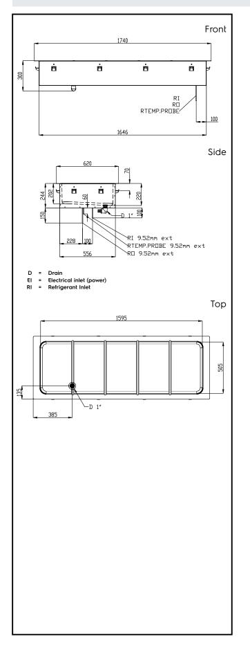
Drop-In Drop-in remote refrigerated well, static (5 GN container capacity)
